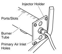
Figure 29 - Injector Holder On Outlet Burner Tube
